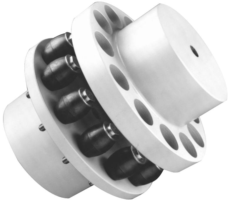
Lovejoy B-FLEX couplings consist of a set of resilient BARREL shaped bushes with pins & nuts and two flanged hubs of graded cast iron.
