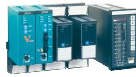
MODEL **1000** For small end DCS applications, Model 1000 consists of one L1 CPU and is capable of up to 8 PID loops, This controller is tag based (MCS style) and has 6k steps of capacity. Features include up to 8 loop display units, Ethernet or Tosline S20LP, which operates on the basis of real time scan transmission, RS485 utilising Computerlink Protocol and the ability to cater for up to 16 process I/O modules.
