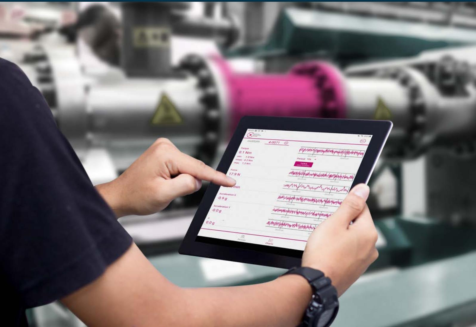
In addition to providing all of the advantages of an R+W coupling, the intelligent coupling system serves as a wireless data source. This is made possible through on-board sensor technology which measures torque, speed and acceleration in addition to special options for axial force and bending moment, all from directly within the rotating drive line.
