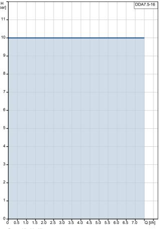
Pumped liquid = Water Liquid temperature during operation = 20 °C Density = 998.2 kg/m³
