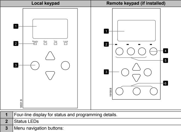
**RESET/EXIT**: Exit the menu or parameter, or cancel a parameter change. On the local keypad, this button also resets a trip.
