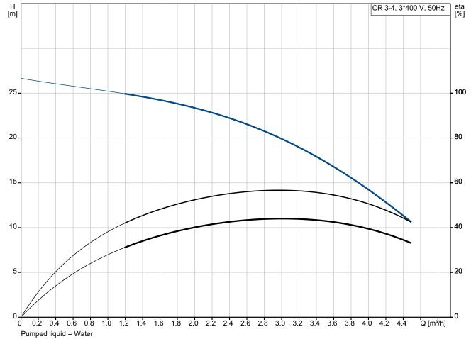
Liquid temperature during operation = 20 °C
