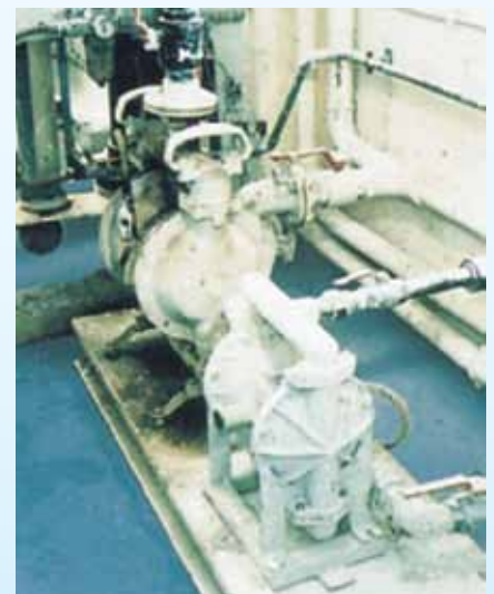
2 Blagdon pumps at Royal Doulton pottery works. The unit at the rear pumped clay slip for 8 years without change of diaphragm, ball valves or valve seats.
