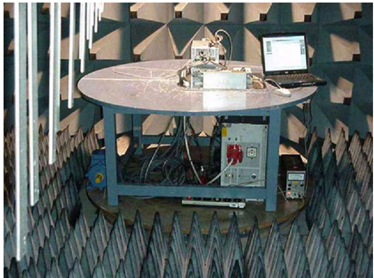
Figure 5.15 RFI voltage and RFI field strength (base without absorber), HF irradiation
