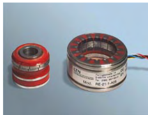
Figure 2.35 Resolver components (source: LTN)
