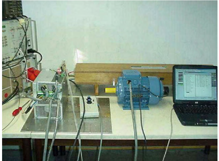
Figure 5.18 Burst on signal and data lines
