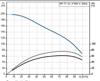
Pumped liquid = Water Liquid temperature during operation = 20  $^{\circ}$ C Density = 998.2 kg/m³
