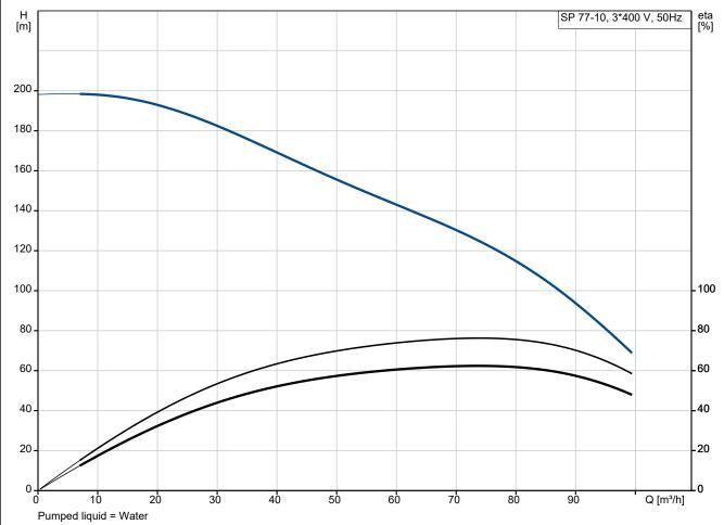
Liquid temperature during operation = 20 °C Density = 998.2 kg/m<sup>3</sup>
