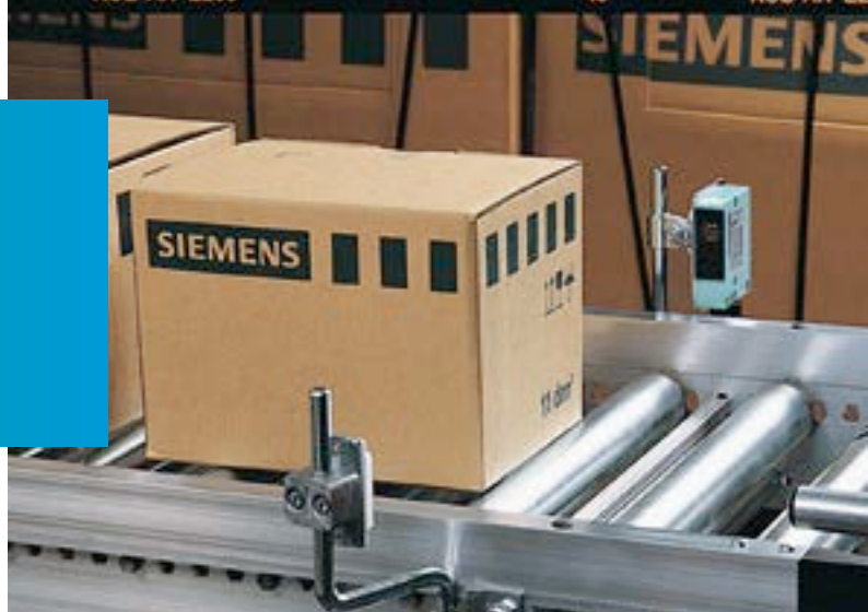
SIRIUS 3RW30 – for soft reversing operation of roller conveyors
