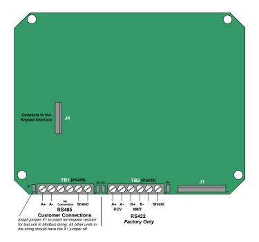
FIG. 2.3.2 RS485 / RS422 Communications Board
