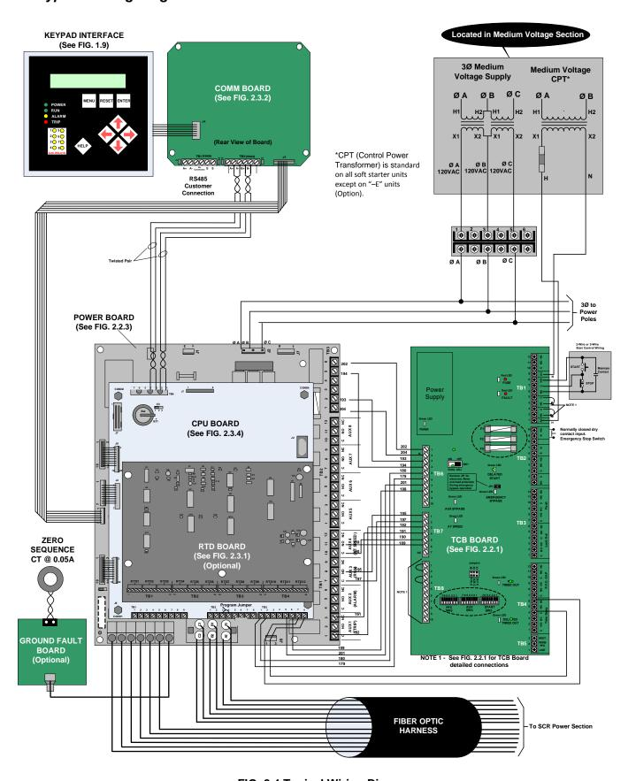
FIG. 2.4 Typical Wiring Diagram
