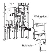
5 Mount the wiring duct in the reverse procedure.First, adjust the bolt hole to the position of the bolt.Be sure to mount the wiring duct before the transparent cover.
