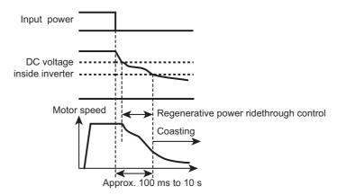
\* Available time to continue the operation varies by the mechanical inertia or load condition. Perform verification test when using this function.
