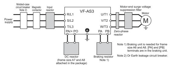
For details of the peripheral devices, refer to [Chapter 10]. **DC reactor**
