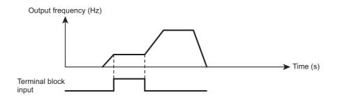
When you set run command ON after you set the dwell operation signal ON, operation will start at <F240: Start frequency>.
