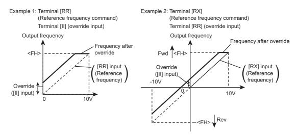
Example 1: <F660>= "3: Terminal II", <F661>= "0: Disabled" Output frequency = Reference frequency + Override (terminal [II] input (Hz))
