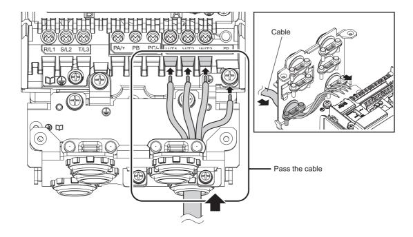
6 Tighten the screws of the terminals [U/T1], [V/T2], and [W/T3] and a terminal [PE]. For the recommended tightening torque, refer to "■Recommended tightening torque of power terminal screws" of [2. 3. 3].
