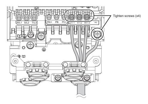
7 Tighten two screws of the cable clamp and fix the motor wiring (four wires) with the cable clamp. The cable clamp exists only in frame size A1 to A5.
