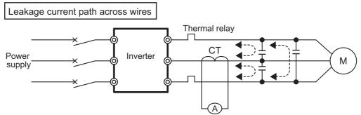
Here are some examples of measures against leakage current across lines.
