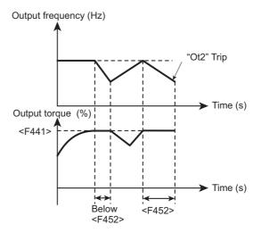
If, during power running, the output torque reaches the value for <F441: Power running torque limit level 1> or more, and continues for the period of time set for <F452: Stall detection time during power running>, the trip "Ot2" will occur. In case F452=0.00, this function is not activated (Ot2 trip does not occur).
