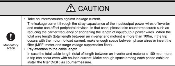
Measures should be taken for leakage current across ground and leakage current between wires because they may cause a malfunction of peripheral device.
