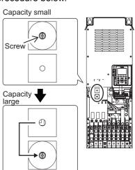
4 After switching, mount the transparent cover and the front cover in this order. For how to mount, refer to [2. 2. 4].
