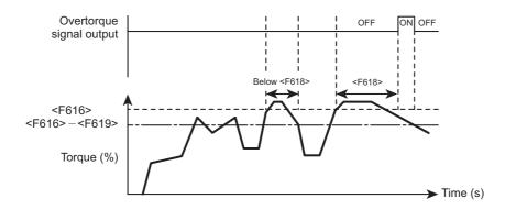
When <F615: Overtorque trip> = "1: Enabled", the inverter trips if overtorque is detected for the period of time specified by <F618: Overtorque detection time>. After that, overtorque (OT) alarm remains ON.
