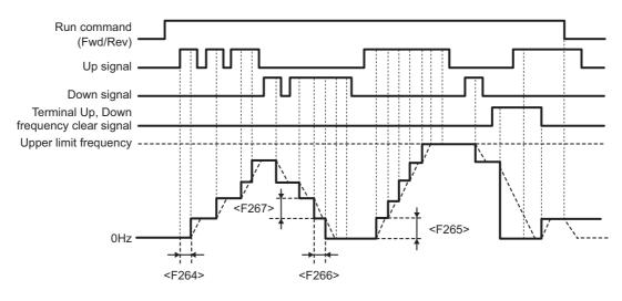
Solid line: Frequency command value Dotted line: Output frequency
