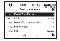
Memo • When you select "1: Rev run" and press the [OK] key, the motor decelerates and starts reverse run. [FWD/REV] key operation is not possible.
