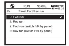
5 Select "2: Fwd run (switchable F/R by panel)" and press the [OK] key.
