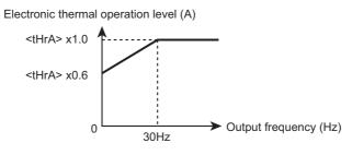
The reduction start frequency of the electronic thermal is fixed to 30 Hz.
