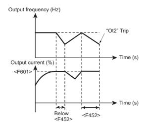
If, during power running, the output current reaches the value for <F601: Stall prevention level 1> or more, and continues for the period of time set for <F452: Stall detection time during power running>, the trip "Ot2" will occur.
