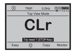
2 When you press the [STOP/RESET] key again while "CLr" is blinking, the trip is reset. The display on the screen once disappears, and the screen immediately after power on is displayed.
