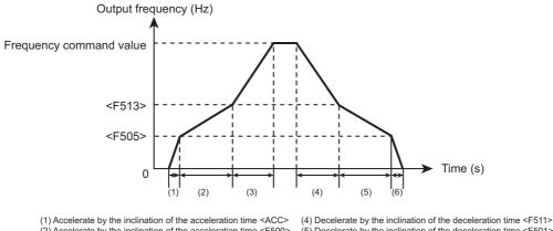
Accelerate by the inclination of the acceleration time <ACC>
