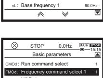
The basic parameter screen is displayed. Check that the setting value of <CMOd: Run command select> is "1."
