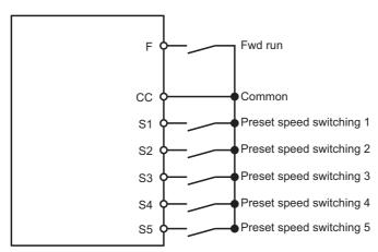
The following is an operation example of preset speed 1 - 3. In this case, set <Sr1: Preset speed 1> to <Sr3: Preset speed 3>.
