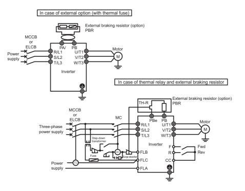
The above connection is for the case where MCCB or ELCB with a trip coil is used instead of MC for TC (trip coil).
