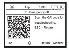
Note) If the camera cannot scan QR code because of the red screen, you can change the backlight color from red to white by pressing the [F2] key.
