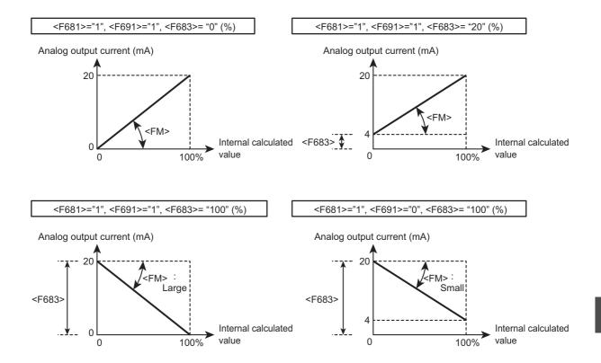
Set the inclination of analog output with <FM: Terminal FM adjustment> and <F671: Terminal AM adjustment>. For details of how to adjust, refer to [5. 2. 6].
