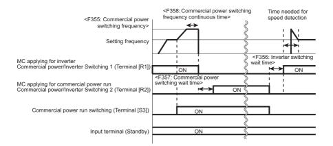
When function numbers "102", "103" (switch to commercial power run) is set to terminal [S3]. Terminal [S3] ON: commercial power operation
