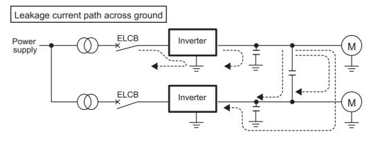
Here are some examples of measures against leakage current across ground.
