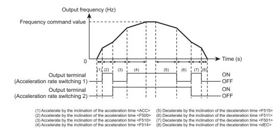
Set run command to terminal run. Set <CMOd: Run command select> to "0: Terminal". Patterns 1 - 4 can be switched by turning the two input terminals ON/OFF. Assign "32: Stall prevention switching/Torque limit switching 1" and "34: Torque limit switching 2" to the two unused input terminals.
