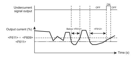
In the case of <F610: Undercurrent trip> = "1: Enabled", when a current is <F611: Undercurrent detection level> or less for the period of time specified by <F612: Undercurrent detection time>, the inverter trips.
