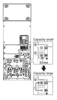
After switching, mount the transparent cover and the front cover in this order.For how to mount, refer to [2. 2. 5].
