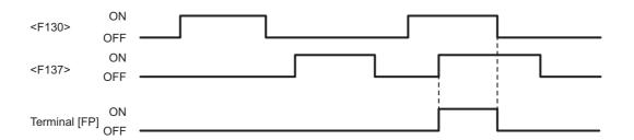
In case of the terminals [R1A]-[R1C], when you set <F139> = "0" or "2", signals are output when the functions set for <F133: Terminal R1 function 1> and <F138: Terminal R1 function 2> are simultaneously turned ON.
