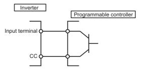
You can connect the input terminal and the terminal [CC] (common) to the programmable controller output (non-logic switch) for control purposes. Use this connecting method for forward/reverse run, or preset speed operation, etc.
