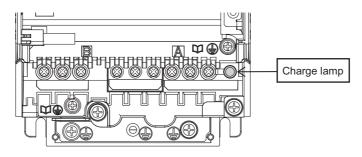
Mount the front cover in the reverse procedure.Pay attention to engagement of the tab and insertion of the upper side of the cover.
