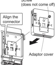
8 Insert a screwdriver, etc. to the lock removal hole of the adaptor cover to push and unlock, and remove the adaptor cover upward. In this state, a cassette option can be inserted to slot C.
