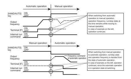
When you do not want to pass on the run/stop state and output frequency under the automatic operation to the manual operation, set <F295> to "0: Disabled".
