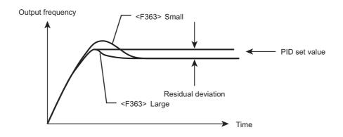
The integral/derivative amount of PID control can be reset with an external signal. Assign function number "52: PID differential/integral reset" to an input terminal.
