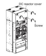
3 Remove the DC reactor cover from the DC reactor by pulling it down.
