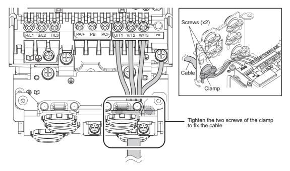
8 Similarly, mount the power supply wiring to the terminals [R/L1], [S/L2], and [T/L3] and a terminal [PE] after passing it through other cable clamp.
