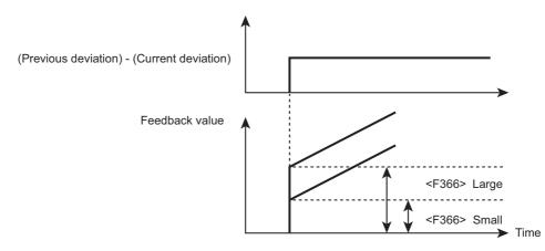
The integral/derivative amount of PID control can be reset with an external signal. Assign "52: PID differential/integral reset" to an input terminal.
