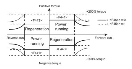
Select from where to input a torque limit value at <F440: Power running torque limit input select 1> and <F442: Regenerative torque limit input select 1>.
