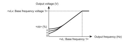
To increase the torque at low speeds, increase the setting value of <vb: Manual torque boost 1>. For details, refer to [5. 3. 6].
