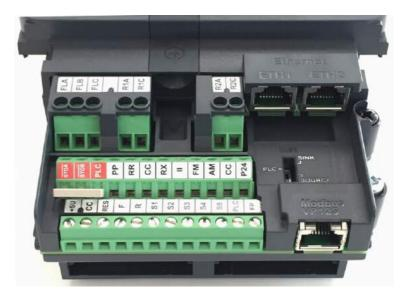
Function setting for the digital input terminals
