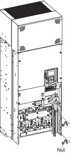
4 Remove the wiring duct from the unit by pulling it down.
