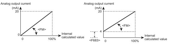
This is when <F682: Terminal FM inclination polarity> is "1: Positive inclination (upward slope)" and <F683: Terminal FM bias> is "0". When<F682> is set to "0: Negative inclination (downward slope)", the inclination becomes negative. This is when <F682> is "1" and <F683: Terminal FM bias> is "20". 20% value (4mA) of the full scale output current (20 mA in this case) will be the output current at internal calculated value of 0%.
