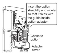
Perform wiring of the cassette option, and then, insert it into slot C straightly and slowly along the guide inside the option adaptor.
