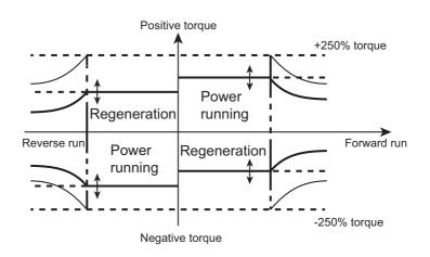
Torque limit value can be changed by external signals.
