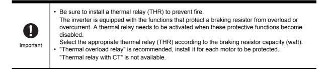
For an application that requires the continuous regenerative state, such as moving down of a lifting gear, press and tension control, or when a deceleration stop is performed for a machine with large load inertial moment, increase the braking resistor capacity according to the operation rate.
