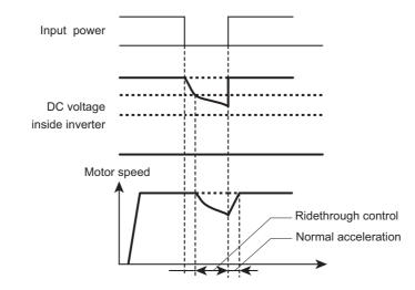
When a momentary power failure occurs during deceleration stop, the regenerative power ridethrough does not function. Setting example of <F302: Regenerative power ride-through> = "2"
