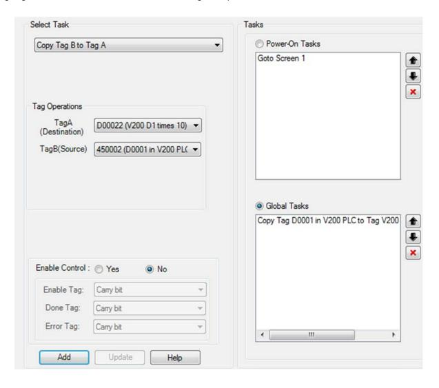
Now D22 can be used as an operand in the multiplication function block above. If a lot of registers from the V200 PLC need to be used in the OIS45E PLUS ladder program, Block Copy is available. A bock of up to 999 continuous registers can be transferred with one Block Copy global task.
