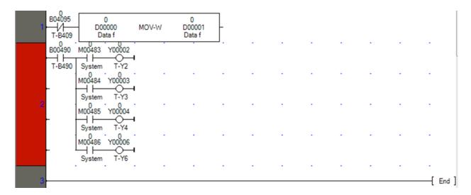
Note: Programming outputs Y00002 thru Y00006 is not necessary. But it does allow confirmation of the special M timing bits in the V200 PLC. These are the same timing bits that control the bit buttons on the OIS45E PLUS.
