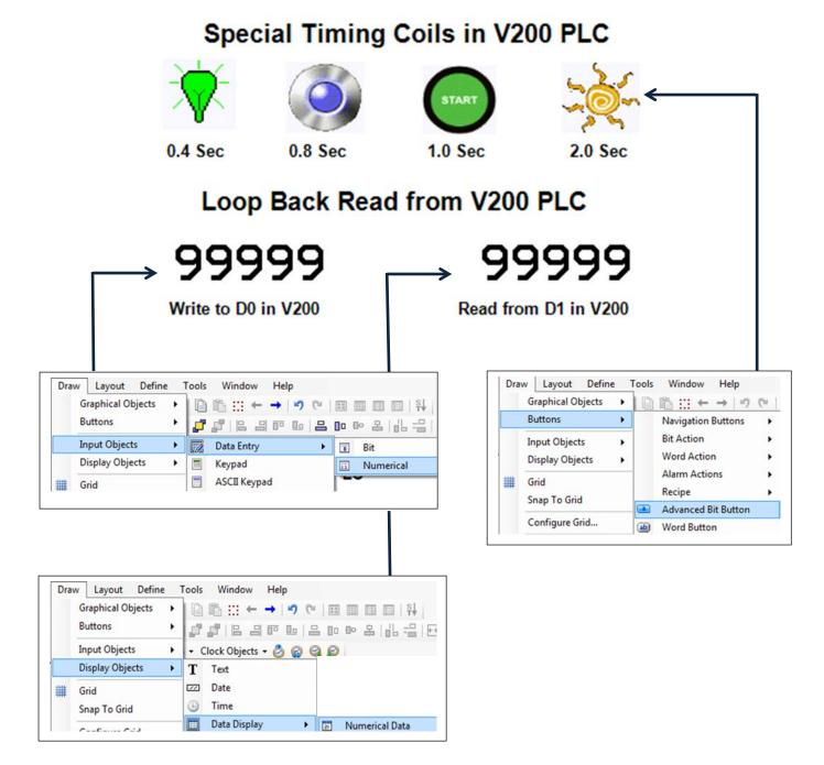
Now the tags can be attached to the screen objects. Often times it is easier to attach the tags to the objects as the objects are created. It can be done either way.
