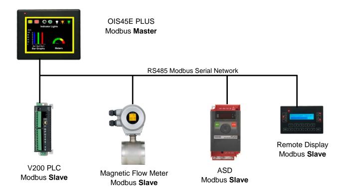
The following example will show how to setup a Modbus master and the Modbus slaves. For simplicity the example will only show setting up the V200 PLC as the Modbus slave. However, setting up the other slaves is very similar.
