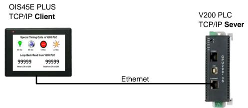
The following Ethernet capable devices, using the OIL-DS software, can be setup as either a Modbus TCP/IP client or a Modbus TCP/IP server:
