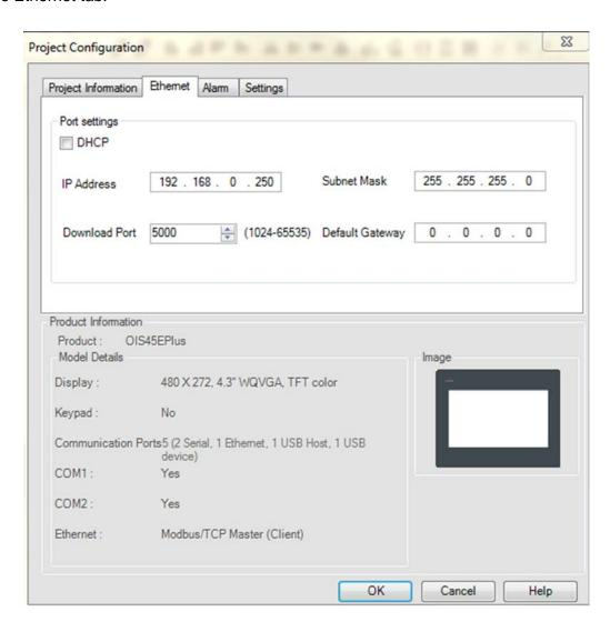
Set the IP Address as shown. Download port should be set at 5000. Accept the defaults for the Subnet Mask and the Default Gateway.
