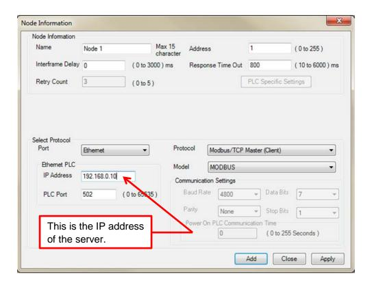
Node 1 is the V200 CPU. Note that it's Ethernet address IP address, 192.168.0 10, is setup here. If additional servers are required, each should be setup as a separate Node with its own Ethernet IP address.
