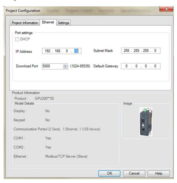
The V200 PLC is now setup as the Modbus TCP/IP server. If additional V200 PLCs are required as servers, they would be setup exactly as above except they would have a different IP address; 192 . 168 . 0 . 20 for example.
