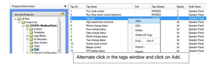
Make sure Node name is Node 1 Modbus RTU (Unit as Master), then enter the Modbus coil 35483 as shown:
