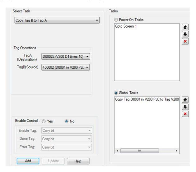
Now D22 can be used as an operand in the multiplication function block above. If a lot of registers from the V200 PLC need to be used in the OIS45E PLUS ladder program, Block Copy is available. A bock of up to 999 continuous registers can be transferred with one Block Copy global task.
