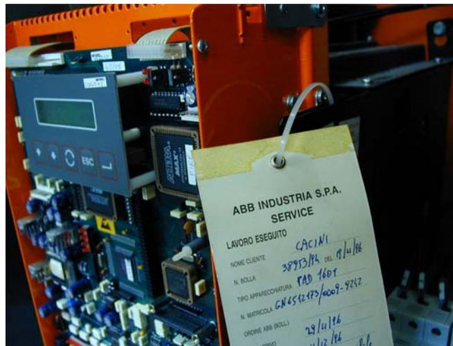
**Regulation rack "REBORN" supply in old Drive ABB e SIEMENS, into a slitter.**
